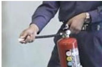
※If you hold the hose in the middle, it may be difficult to aim accurately due to the pressure during discharge.
